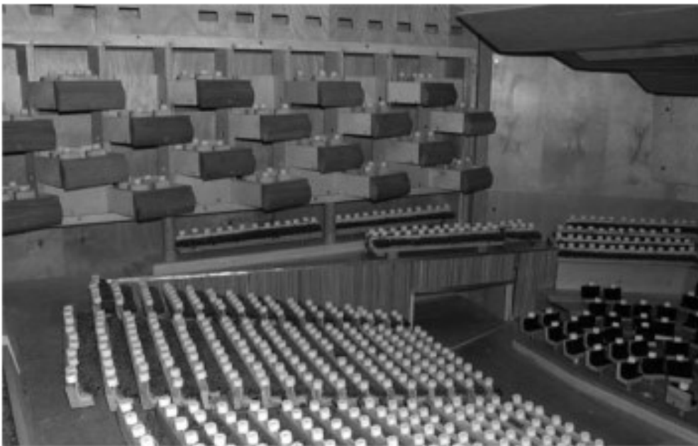
Figure 8.5 Physical model: acoustic model of a concert hall (© Kirkegaard Associates)
